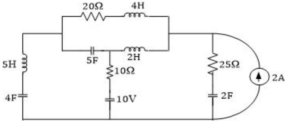
For the network shown in Figure below, obtain network equilibrium equations on node basis using KCL.
